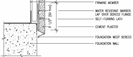
Weep Screed at Concrete Foundation
