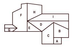
B. Sketch a diagram of each roof section. Show all measurements (see example below.) It is important to measure exact center of the ridge to the eave edge. Do not allow anything for overhang.
