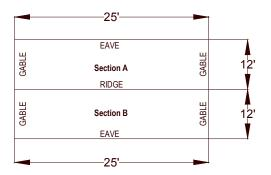
The length from the eave to the ridge is 12'. The length of the ridge is 25'; therefore, the number of panels to complete one side of the house is  $25 \div 3 = 9$  pcs. Your materials list should look like Sample "B" on page 9.
