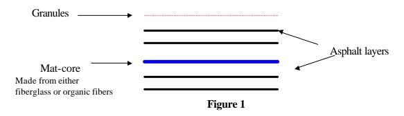
Asphalt shingles are manufactured with either a fiberglass mat-core or an organic mat-core.
