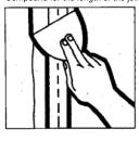
with 125 mm (5") finishing knife. Centre and lightly press CGC Drywall tape into the wet drywall compound with fingers. Starting near the centre of the joint, draw 125 mm (5") knife
