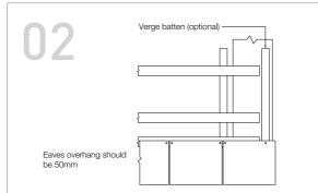
Set out both under-eaves battens to accommodate the two lengths of under-eaves slates (Table 6, page 21) allowing for correct lap and gauge. Cut the under-eaves slates from a standard slate and drill 2 no. 4mm dia. holes approximately 10-15mm in from the top cut edge and head nail the first under-eaves course along the eaves.
