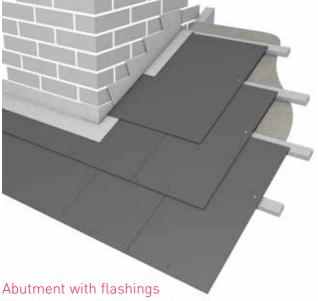
Where slates abut walls, chimney stacks, rooflights and dormer windows, etc., the jointing should be weathered by conventional lead soakers and flashings.
