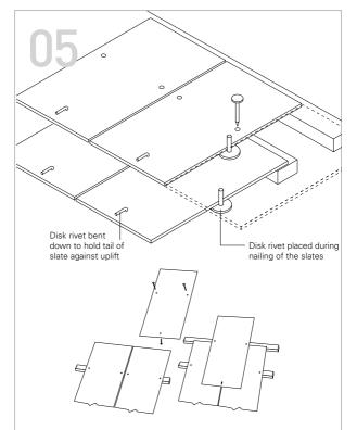
To achieve the correct bend in the rivet pin, it is best to tap it twice with a hammer, once at about 45° to the pin, and then finally onto the surface of the slate.
