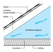
Cold pitched roof with type HR underlay, ventilated void above insulation and a well sealed ceiling
