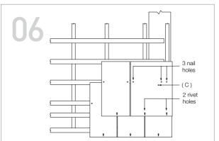
At verges and abutments, lay the first full length slate-and-a-half slate, ensuring that 3 no. 4mm dia. holes are drilled on the batten line with 2 no. additional holes for the copper disc rivets.
