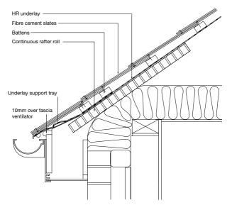
\* If an LR underlay is used, then 25mm counterbattens are required.
