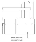
Cut and nail fix second under-eaves course to the lower eaves batten with slate-and-a-half widths at the verge, ensuring a copper disc rivet is fitted centrally between adjacent slates (5mm gap) to align the pin with the hole in the front edge of the first course of full length slates.
