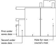
At the verge, a second hole (4mm dia.) is required to allow for the copper disc rivet for the next course. This is drilled 50mm from the outside edge of the slate and 25mm plus gauge from the bottom edge or tail.
