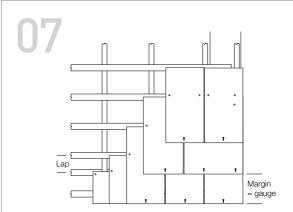
Continue diagonally up the roof with standard size slates, trimming to verges, hips, valleys and ridges as required. Slate-and-a-half widths should be used if the half slate is less than 150mm wide.
