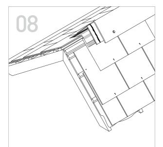
At the roof apex or top abutment, an additional top course batten is fitted directly above the last full length slate batten. The last full length roof slates/short courses are cut to length so that their top edges rest on the lower batten and are centre nailed as normal.
