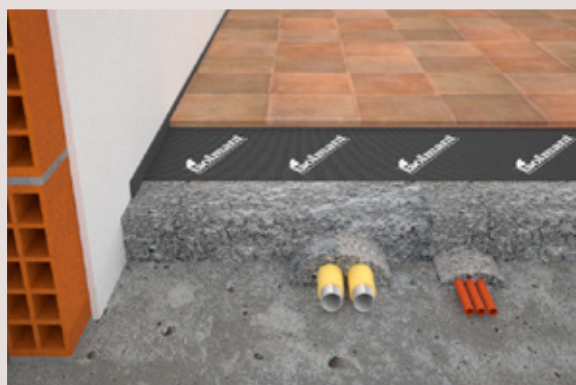
Base slab Levelling screed Isolmant IsolTile Finishing
