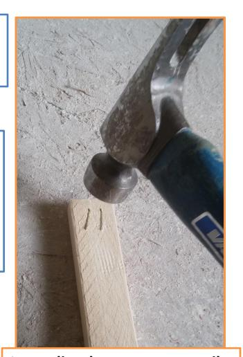
Immediately remove any nails sticking out of this board and bend over any staples.
